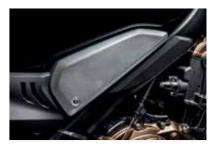
SIDE COVERS 08F75-MKN-D50 High quality aluminium left and right panels that will cover the side of the bike.
