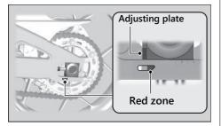
Drive Chain ► Checking the Drive Chain Slider
