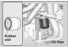
**8.** Apply a thin coat of engine oil to the rubber seal of a new oil filter.
