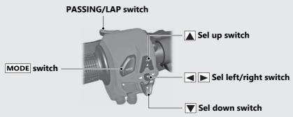
When switching or setting the display, refer to the switch operation guide is displayed.
