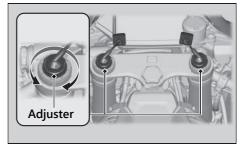
**4.** Turn clockwise to increase spring preload (hard), or turn counterclockwise to decrease spring preload (soft).
