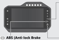
PGM-FI (Programmed Fuel Injection) malfunction indicator lamp (MIL)
