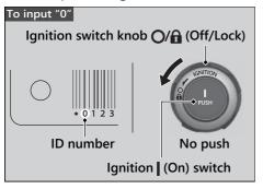
To input "1", push the ignition I (On) switch once, and then turn the ignition switch knob O/A (Off/Lock) counterclockwise to input the next digit.
