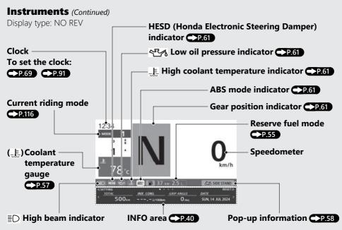
The tachometer is not displayed when NO REV is selected.
