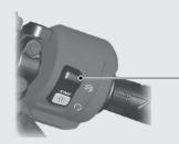
**Engine stop switch/** (3) **Start button** Should normally remain in the (Run) position.
