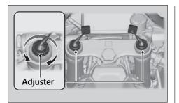
**4.** Turn clockwise to increase spring preload (hard), or turn counterclockwise to decrease spring preload (soft). The standard position is the 2 turns from the full soft position.
